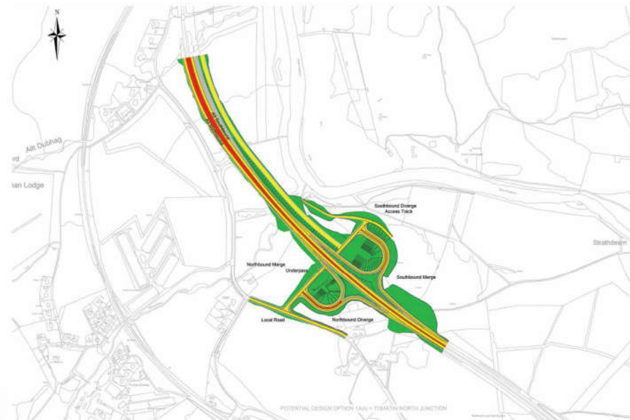
Tomatin North grade-separated junction
