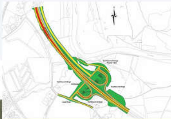
Tomatin North grade-separated junction
