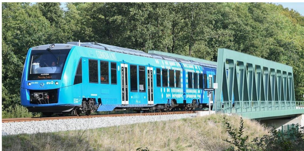
Alstom iLint hydrogen fuel cell powered train, Lower Saxony 2019
