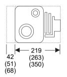
The camera tile is extended on the left by 42 (51) (68) mm (4.5 sw), then the resulting assembly is centred horizontally on the sign.
