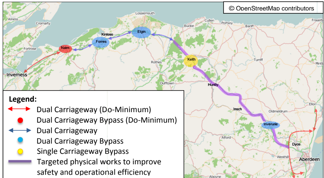
Figure 4-5: Option 5: Bypasses and dualling of heavily trafficked sections plus targeted trunk road improvements
