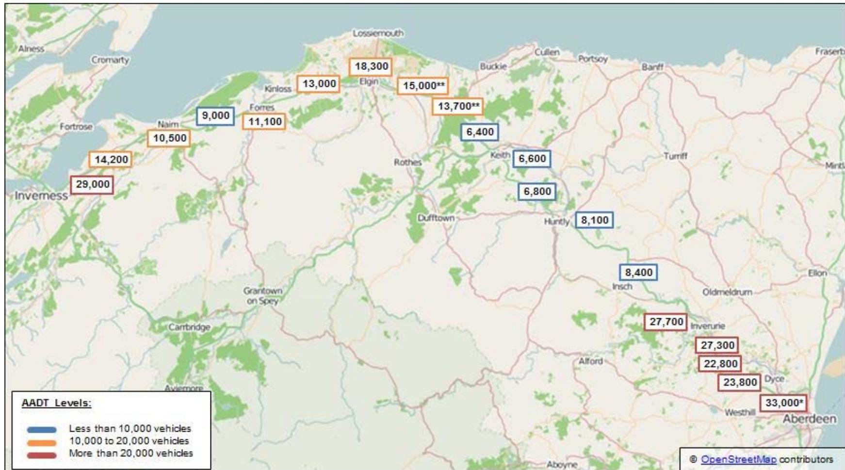
Figure 2-6: Annual Average Daily Traffic by Section in 2012 (2011*) (2010**) from Scottish Road Traffic Database, Transport Scotland
