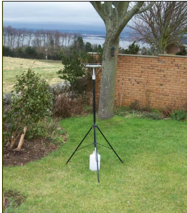
Figure 1: Example of an Installed Frisbee Gauge Meter
