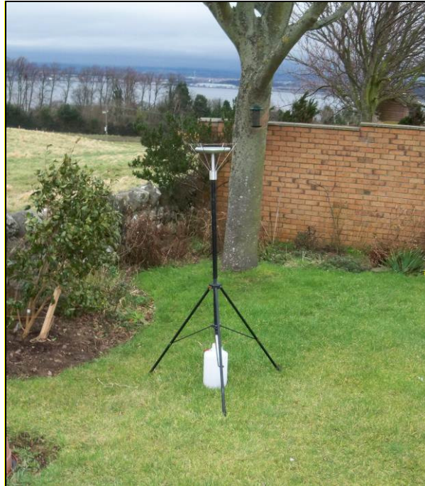
Figure 1: Example of an Installed Frisbee Gauge Meter
