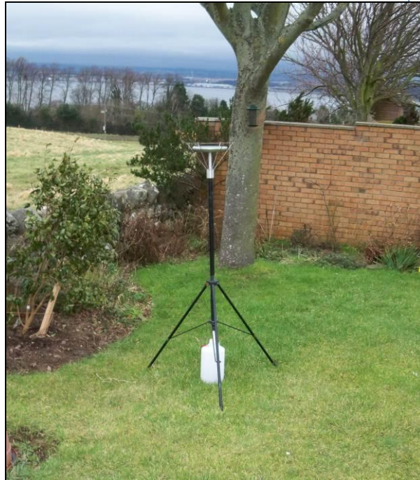
Figure 1: Example of an Installed Frisbee Gauge Meter
