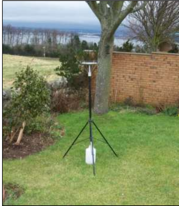
Figure 1: Example of an Installed Frisbee Gauge Meters
