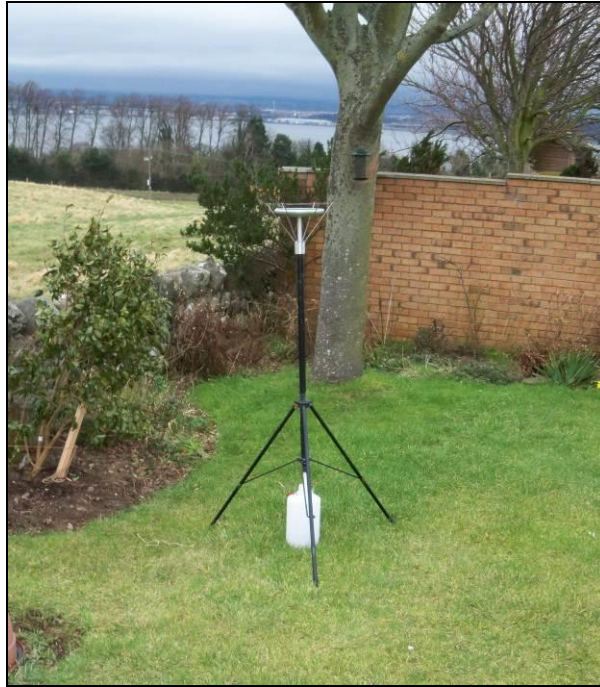
Figure 1: Example of an Installed Frisbee Gauge Meter
