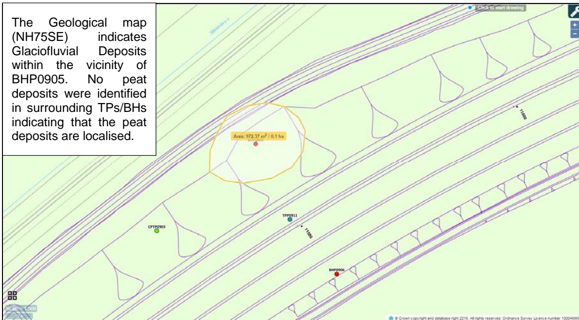
Diagram 1.3: Estimated area of soft deposits to be addressed at Culblair
