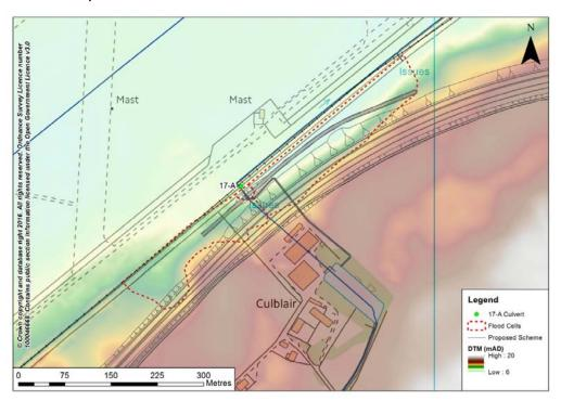
4.44 The flood cells have been defined by the ground topography and the connection ('spill') between adjoining cells is represented by the ground topography along the flood cell boundary.
