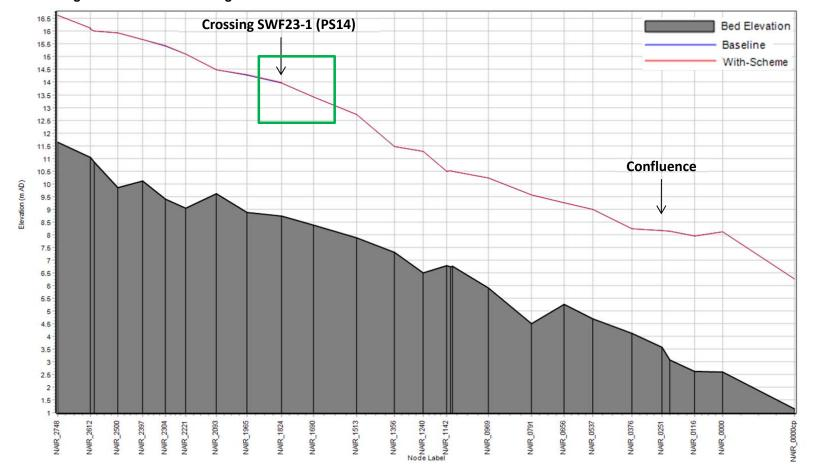
Diagram A1: River Nairn Long Section – 0.5% AEP +CC Event - In-Channel Peak Water Levels
