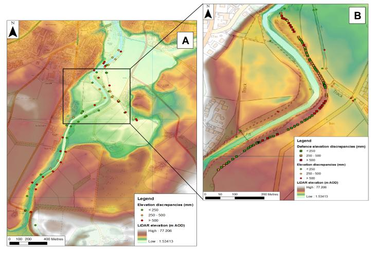
(A) Channel cross section survey, bank top level comparison.
