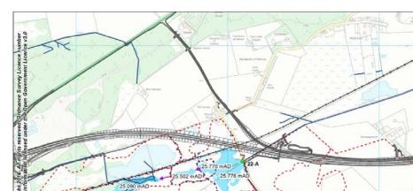
Diagram 4.14: Scheme flood map for the design flood event.
