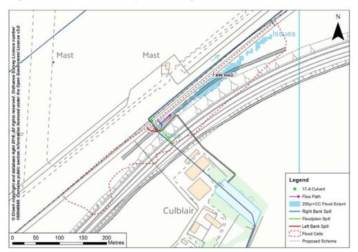
Diagram 4.10: Scheme flood map for the design flood event
