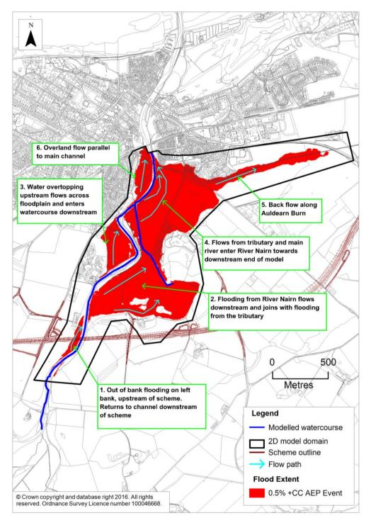
Diagram 13: 0.5% AEP +CC Event Flood Mechanisms
