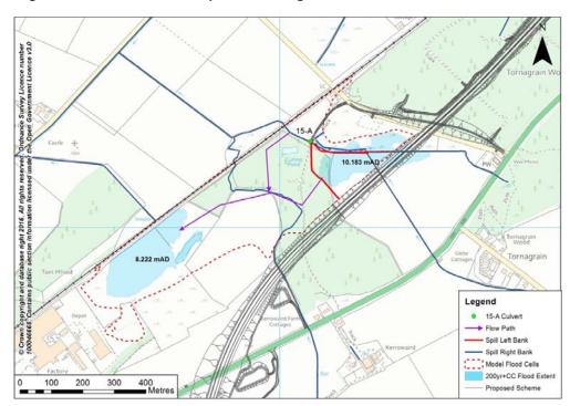
Diagram 4.7: Scheme flood map for the design flood event.
