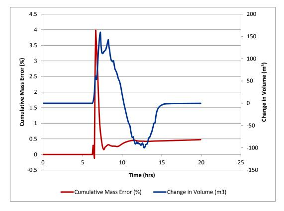
Diagram 6: 2D Cumulative Mass Error and Change in Volume – 0.5 % AEP Event
