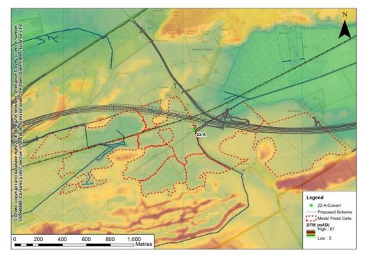
4.57 The flood cells have been defined by the ground topography and the connection (spill) between adjoining cells is represented by the ground topography along the flood cell boundary.
