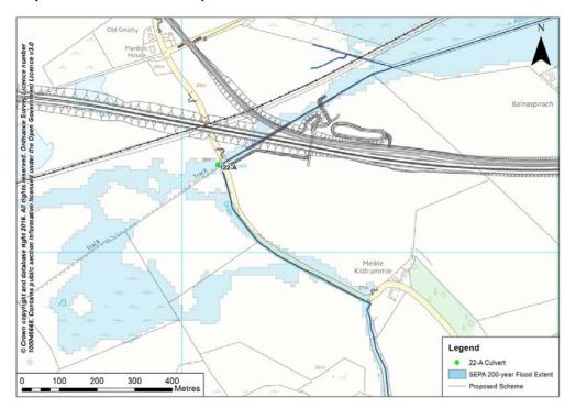
4.55 Further hydraulic assessment has been undertaken, to investigate the impact of road construction on flood risk. This has involved derivation of a simple routing model, based on an inflow hydrograph for the design flood event, representation of the ground topography and existing hydraulic controls.
