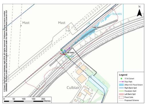
4.47 The forward passage of water is restricted by an existing downstream 0.7m x 0.9m box culvert, which results in floodwater spilling out of bank to the right hand floodplain. The predicted peak water level at this location is 7.47mAOD and the flood extent extends laterally parallel to the railway line for approximately 300m. The flood extent reaches the toe of the proposed road embankment.
