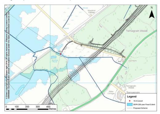
4.19 Further hydraulic assessment has been undertaken, to investigate the impact of road construction on existing flood risk. This has involved derivation of a simple routing model, based on an inflow hydrograph for the design flood event, representation of the ground topography and existing hydraulic controls.
