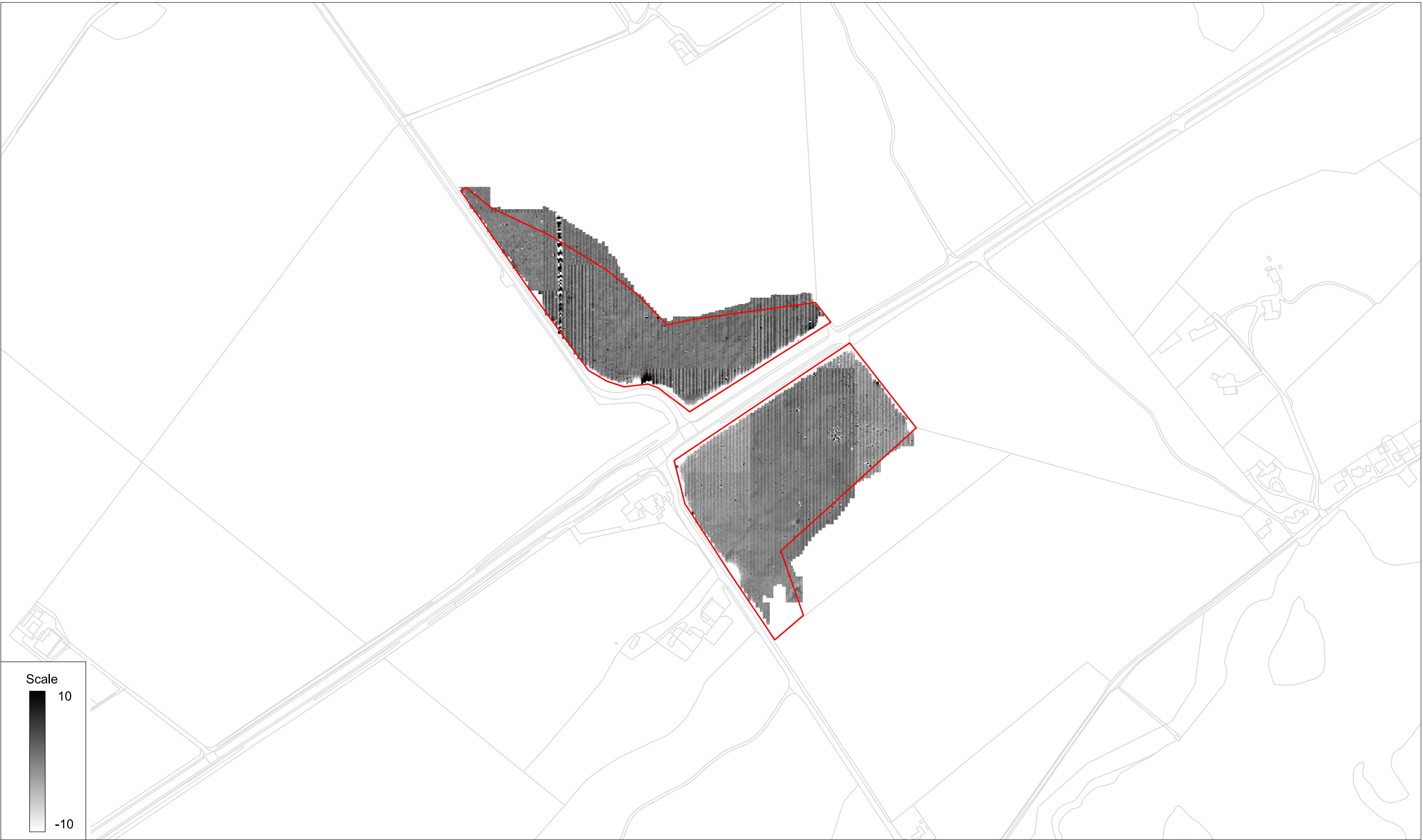
Unprocessed gradiometer survey results greyscale plot: parcel 9
