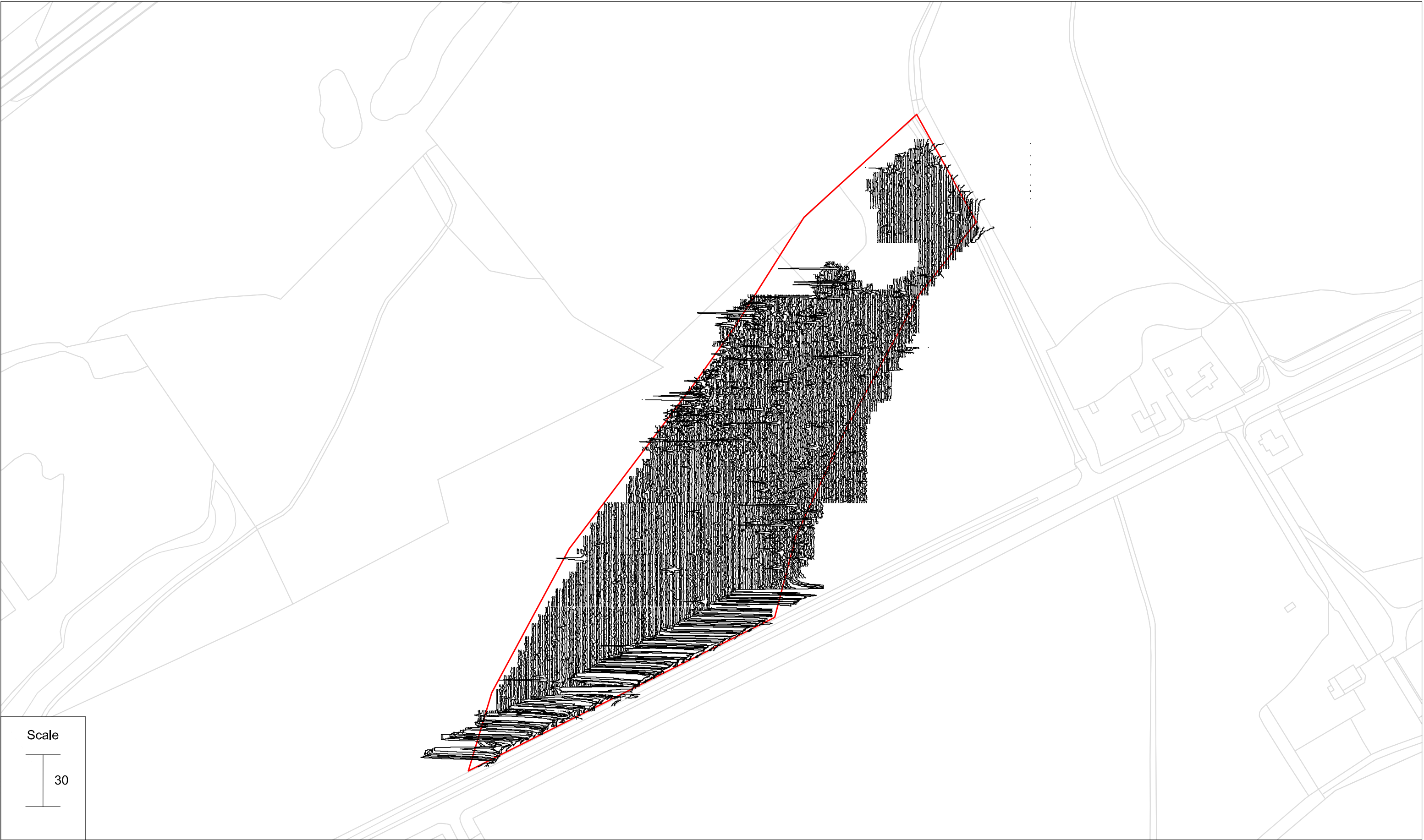
Minimally processed gradiometer survey results xy trace plot: parcel 6
