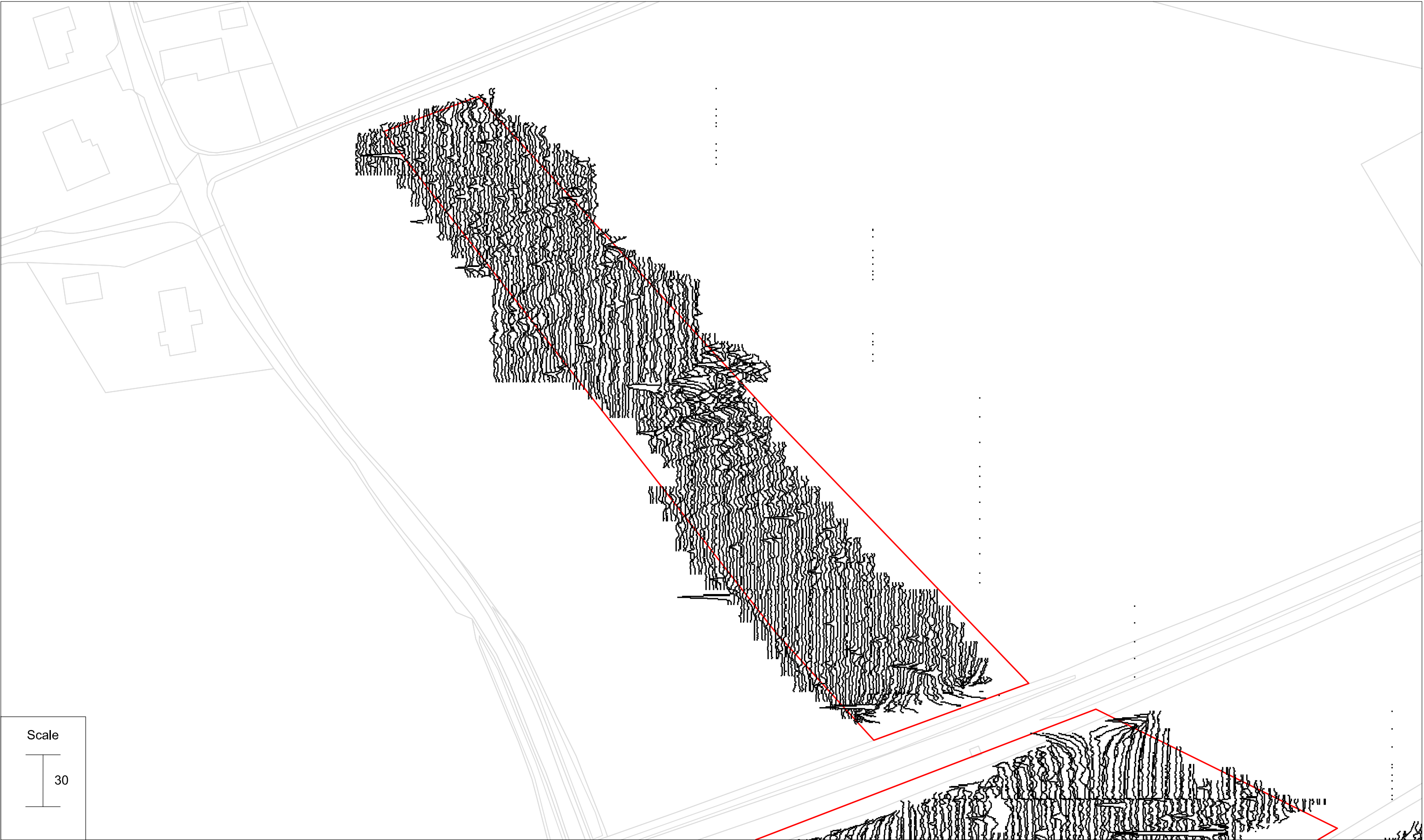
Minimally processed gradiometer survey results xy trace plot: parcel 12a
