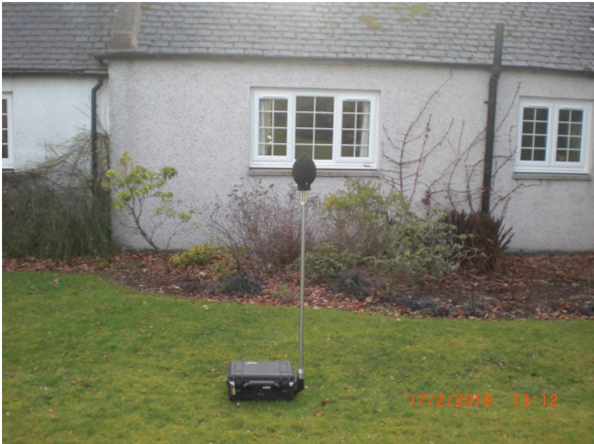
Photograph 22: Noise Monitoring Equipment at East Lodge Cottage
