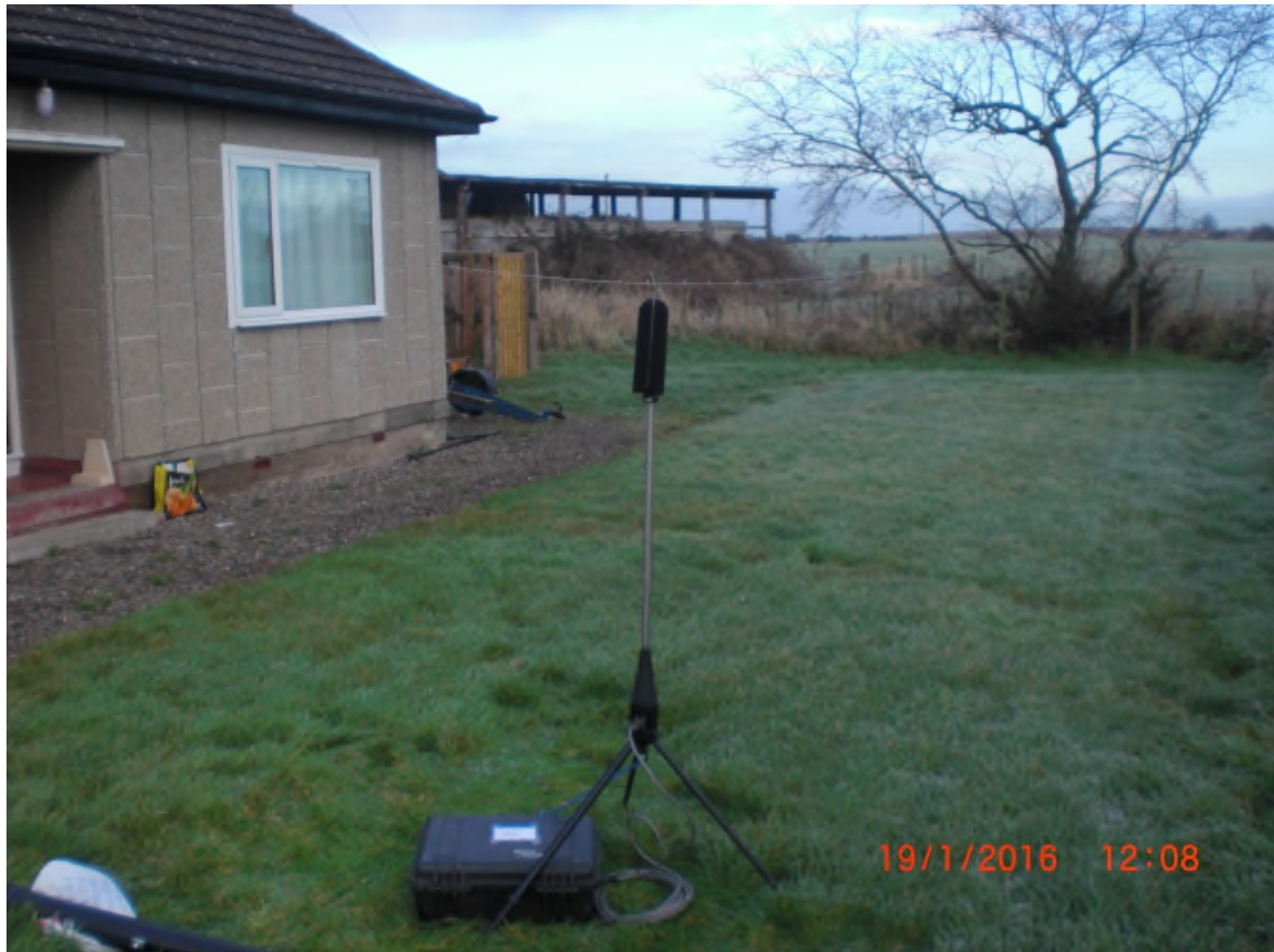
Photograph 4: Noise Monitoring Equipment at The Bungalow
