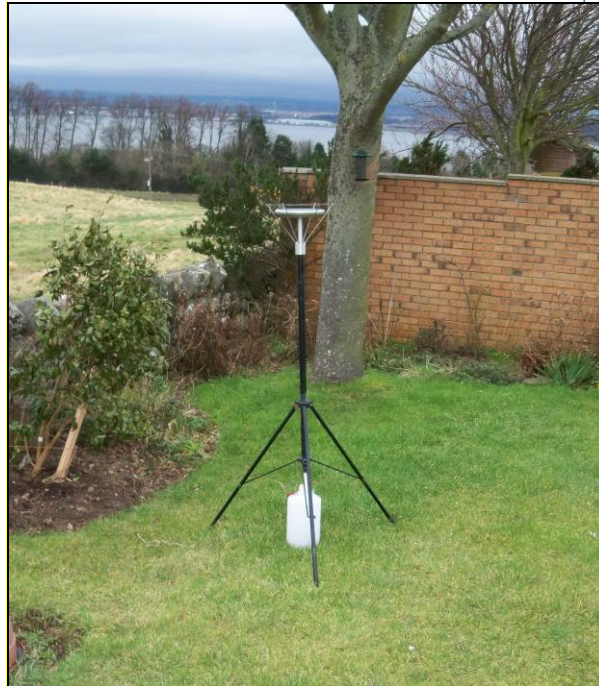
Figure 1: Example of an Installed Frisbee Gauge Meter
