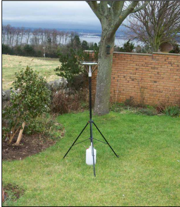
Figure 1: Example of an Installed Frisbee Gauge Meters
