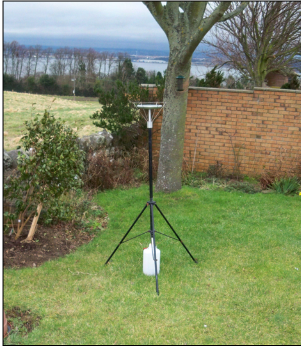
Figure 1: Example of an Installed Frisbee Gauge Meters
