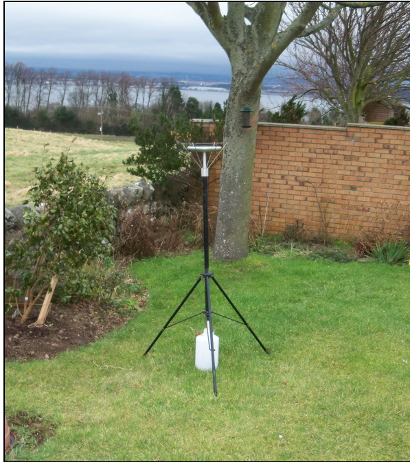
Figure 1: Example of an Installed Frisbee Gauge Meters
