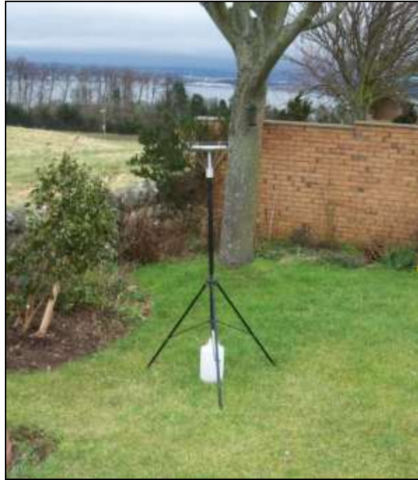
Figure 1: Example of an Installed Frisbee Gauge Meters
