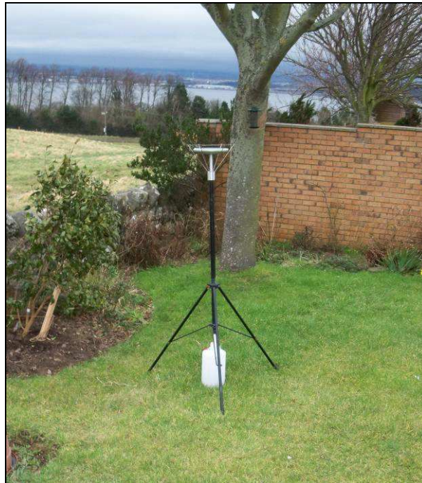
Figure 1: Example of an Installed Frisbee Gauge Meter
