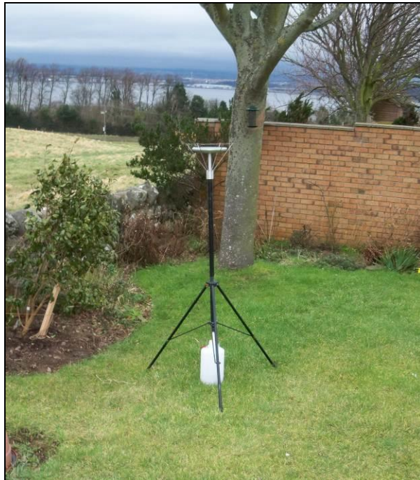
Figure 1: Example of an Installed Frisbee Gauge Meter
