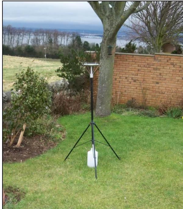
Figure 1: Example of an Installed Frisbee Gauge Meter
