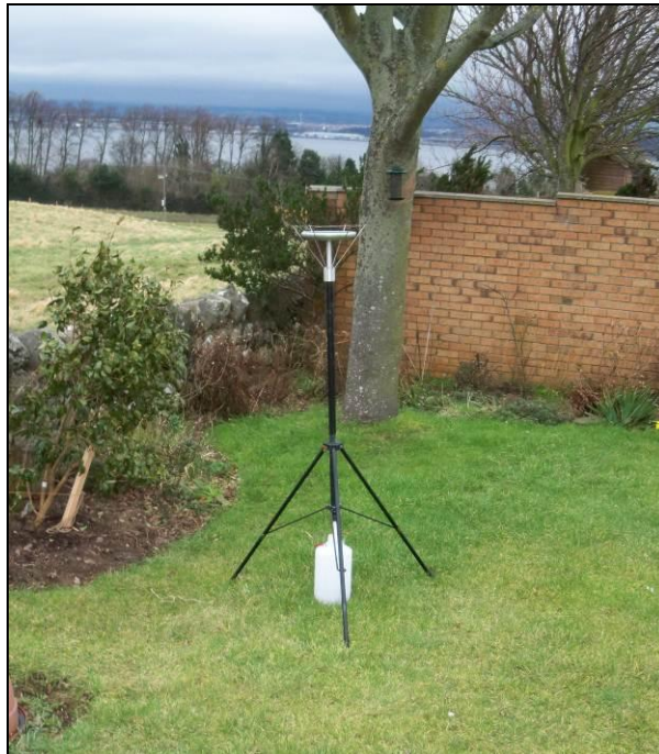
Figure 1: Example of an Installed Frisbee Gauge Meter
