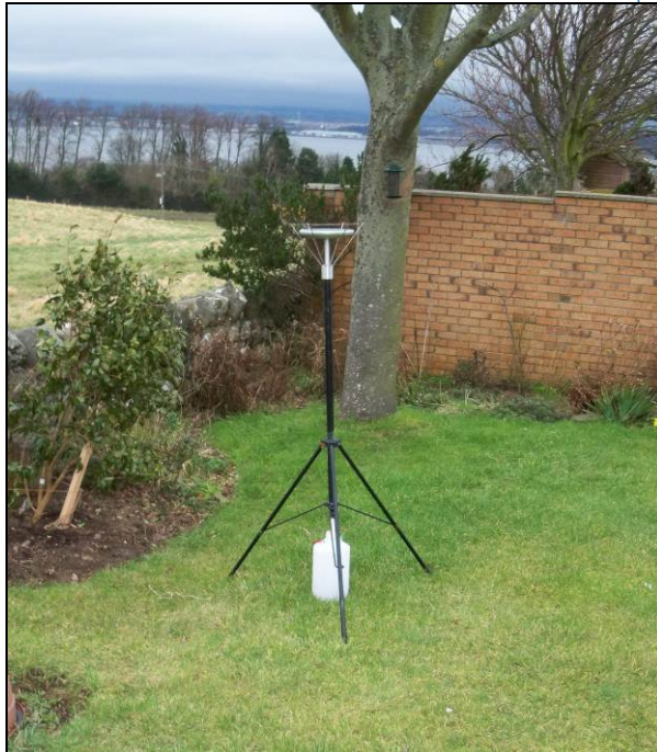
Figure 1: Example of an Installed Frisbee Gauge Meter
