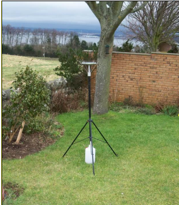
Figure 1: Example of an Installed Frisbee Gauge Meter
