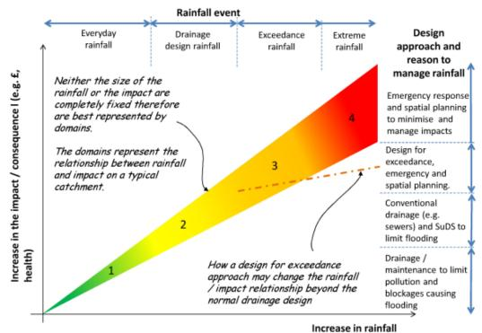
*Figure 4-3: The 4 domain approach showing how designing for exceedance fits into the design process (CIRIA RP991)*
