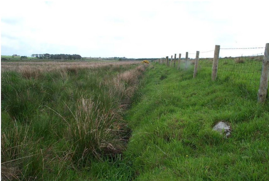
NO8717196299: View downstream at location of proposed road crossing. Grasses/sedges in channel, boggy ground, no perceptible flow.
