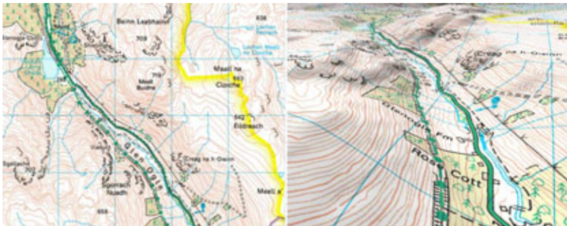
Ordnance Survey mapping for Glen Ogle, presented conventionally in two-dimensions (left) and in draped over a digital elevation model (right) to illustrate relative heights. (© Crown Copyright. All rights reserved Scottish Government 100020540, 2008.)
