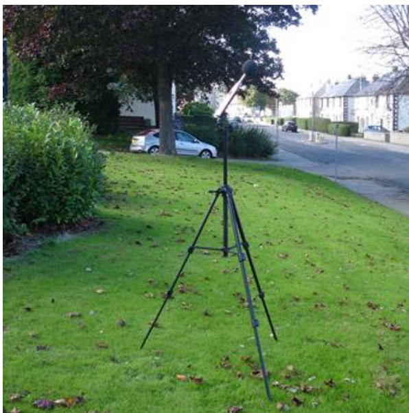
Baseline noise monitoring
