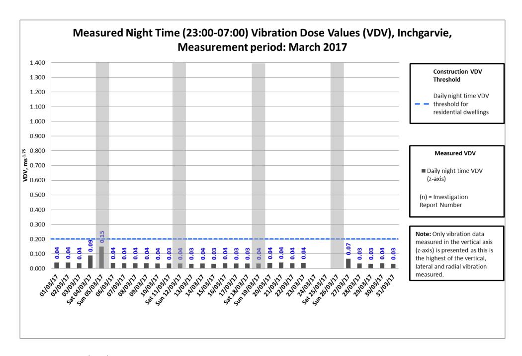
Data missing on the  $24^{th} - 26^{th}$  March was caused by electrical issue with monitor.
