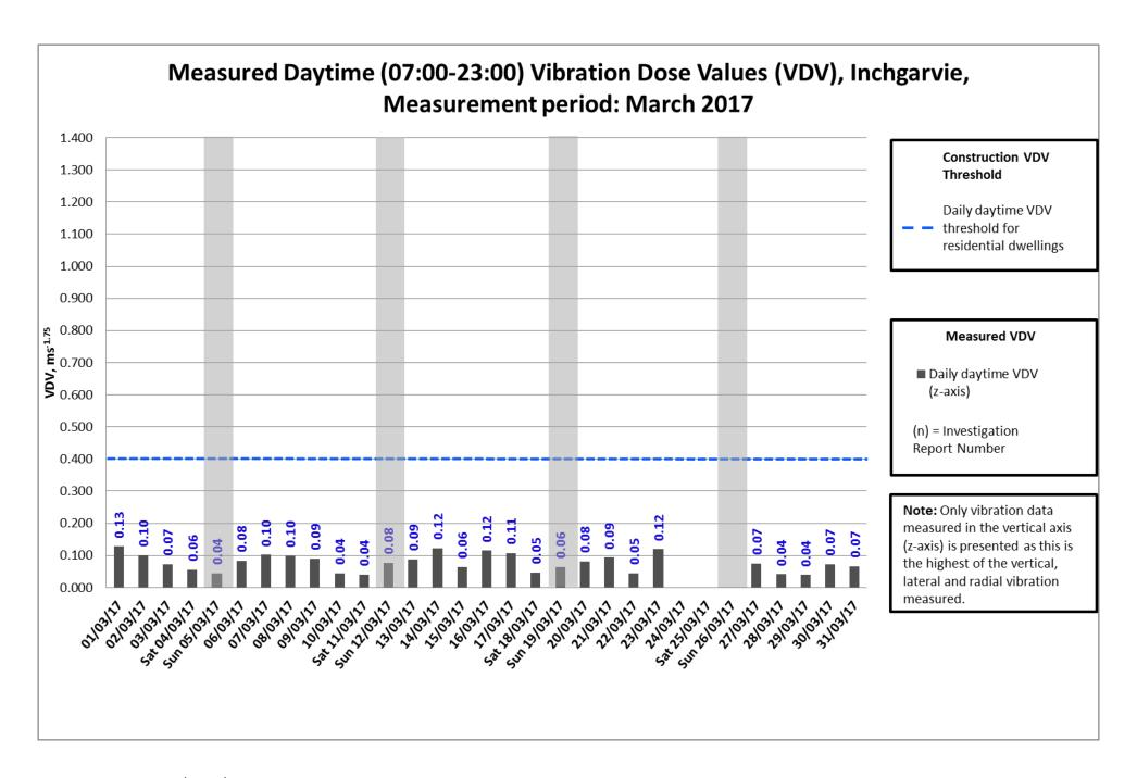
Data missing on the 24<sup>th</sup> – 26<sup>th</sup> March was caused by electrical issue with monitor.
