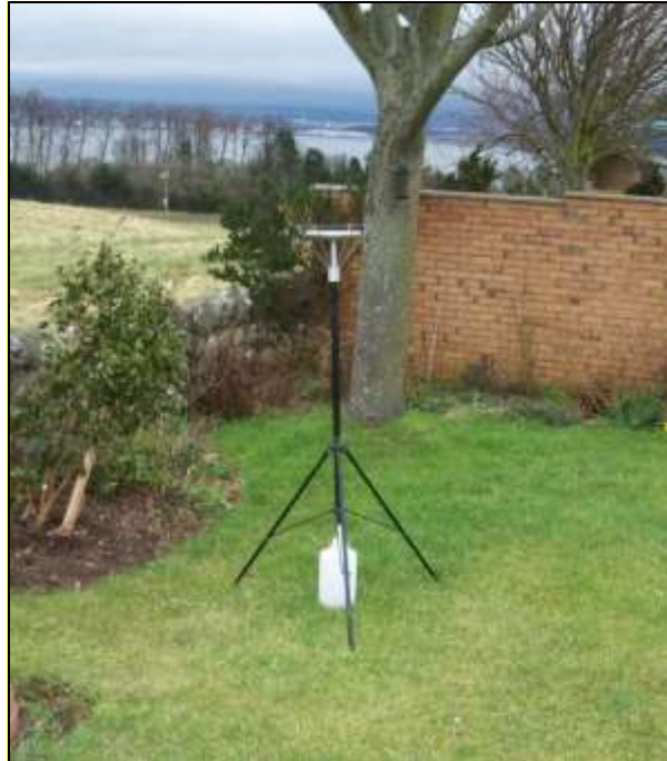
Figure 1: Example of an Installed Frisbee Gauge Meter
