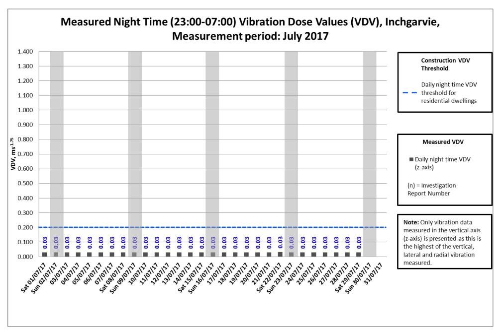
Data missing on the  $30^{th} - 31^{st}$  of July caused by electrical issue with monitor
