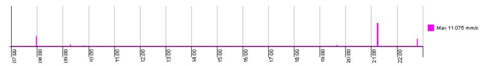
Exceedances on the 5<sup>th</sup>, 6<sup>th</sup>, 25<sup>th</sup> and 26<sup>th</sup> of July have been investigated and found to be caused out with construction working hours therefore it is unlikely that a construction related activity was the cause of these events (graph above from the 05/07/2017).
