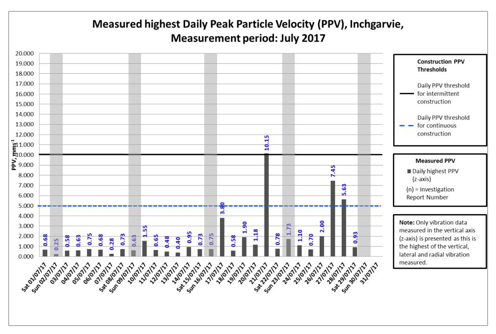
Data missing on the  $30^{th} - 31^{st}$  July caused by electrical issue with monitor
