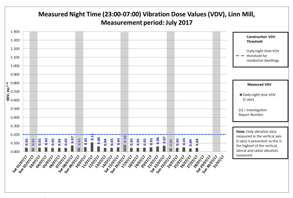
Data missing on the 28<sup>th</sup> – 31<sup>st</sup> of July caused by electrical issue with monitor
