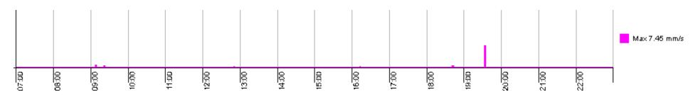
Exceedance on the 27<sup>th</sup> of July has been investigated and found to be caused out with construction working hours therefore it is unlikely that a construction related activity was the cause of this event (graph above from the 27/07/2017).
