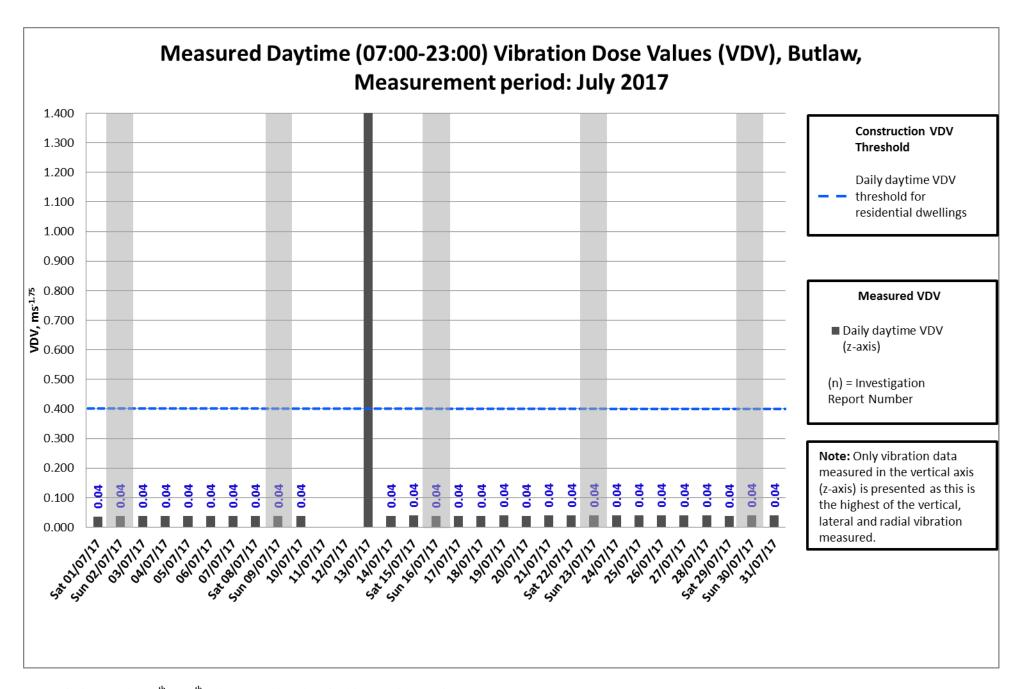
Data missing on the 11<sup>th</sup> – 12<sup>th</sup> July caused by electrical issue with monitor
