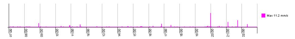
Exceedances on the 24th and 25<sup>th</sup> of July have been investigated and found to be caused out with construction working hours therefore it is unlikely that a construction related activity was the cause of these events (graph above from the 24/07/2017).
