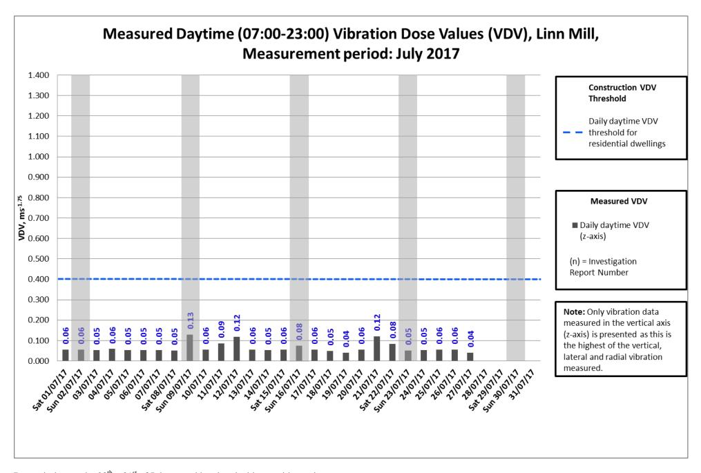
Data missing on the  $28^{th} - 31^{st}$  of July caused by electrical issue with monitor
