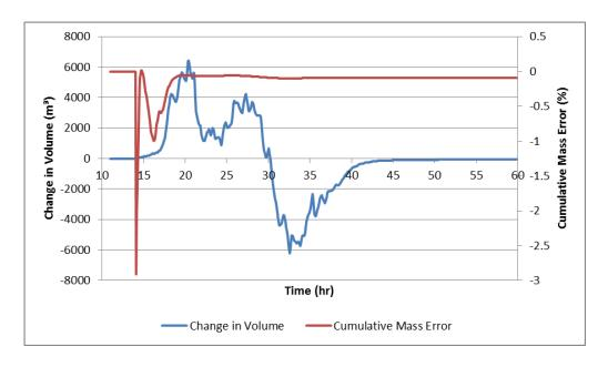
Diagram 19: Cumulative mass error and change in volume Model VI 0.5% AEP plus CC Event
