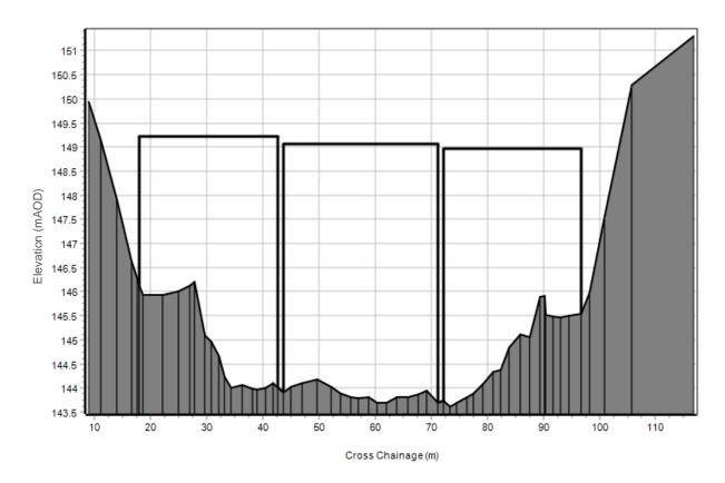
Diagram 7: Pitaldonich Underbridge 1D schematisation in Flood Modeller
