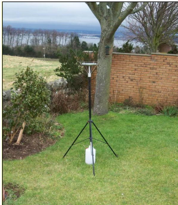
Figure 1: Example of an Installed Frisbee Gauge Meter
