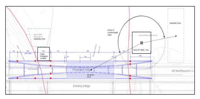
Figure 2: Option 2 for Construction of Tummel Underbridge (Indicative). Red crosses are indicative vertical support positions.
