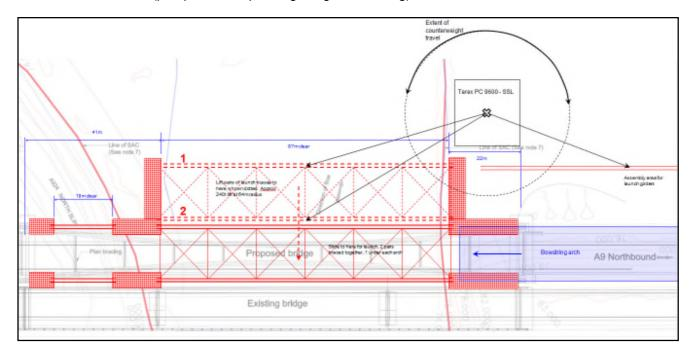
Figure 1: Option 1 for Construction of Tummel Underbridge (Indicative). Red hatching shows indicative footing areas.
