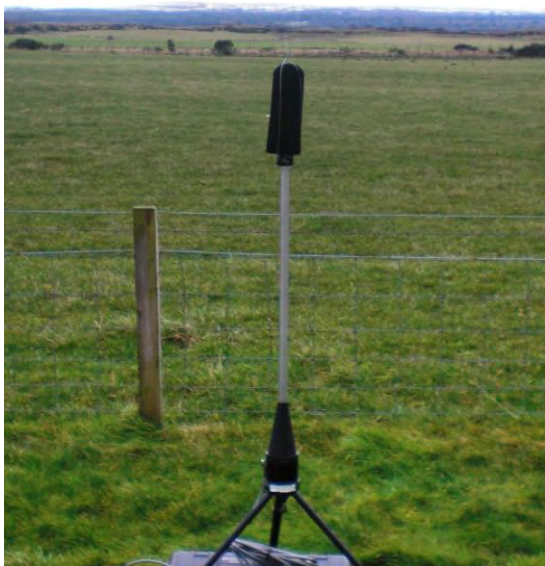
Photograph 11: Baseline noise monitoring equipment
