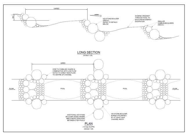
Figure 5-11: Schematic overview of typical cascade with pools detail
