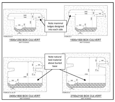
Figure 5-10: Typical cross-sections of buried box culverts with bed material and mammal ledges
