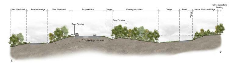
Cross Section E-E' (ch.7550) Scale 1:500
