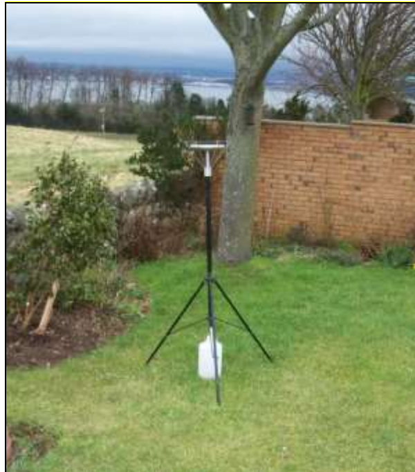
Figure 1: Example of an Installed Frisbee Gauge Meter
