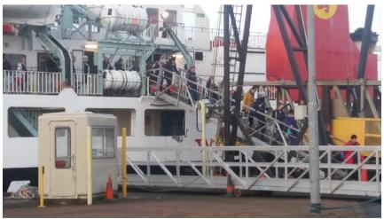
Photo 1. The gangway at Ardrossan showing a 45 of angle, which is extremely difficult for disabled travellers to negotiate.
