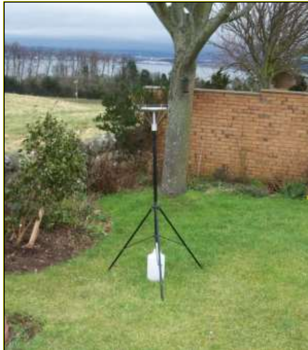
Figure 1: Example of an Installed Frisbee Gauge Meter
