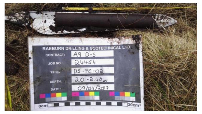
Figure 12. Peat Core DS-PC-02 taken at depth 2.0 – 2.4m
