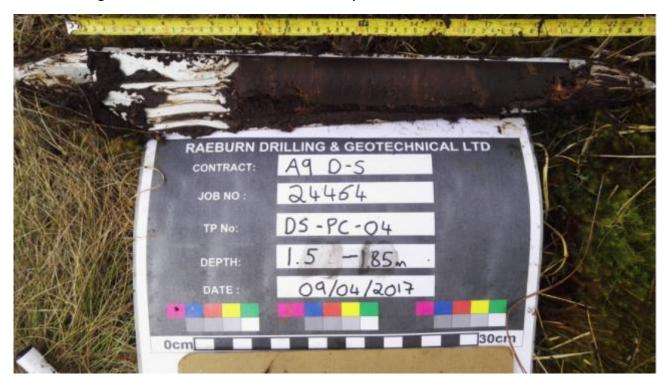
Figure 17. Peat Core DS-PC-04 taken at depth 1.5 – 1.85m
