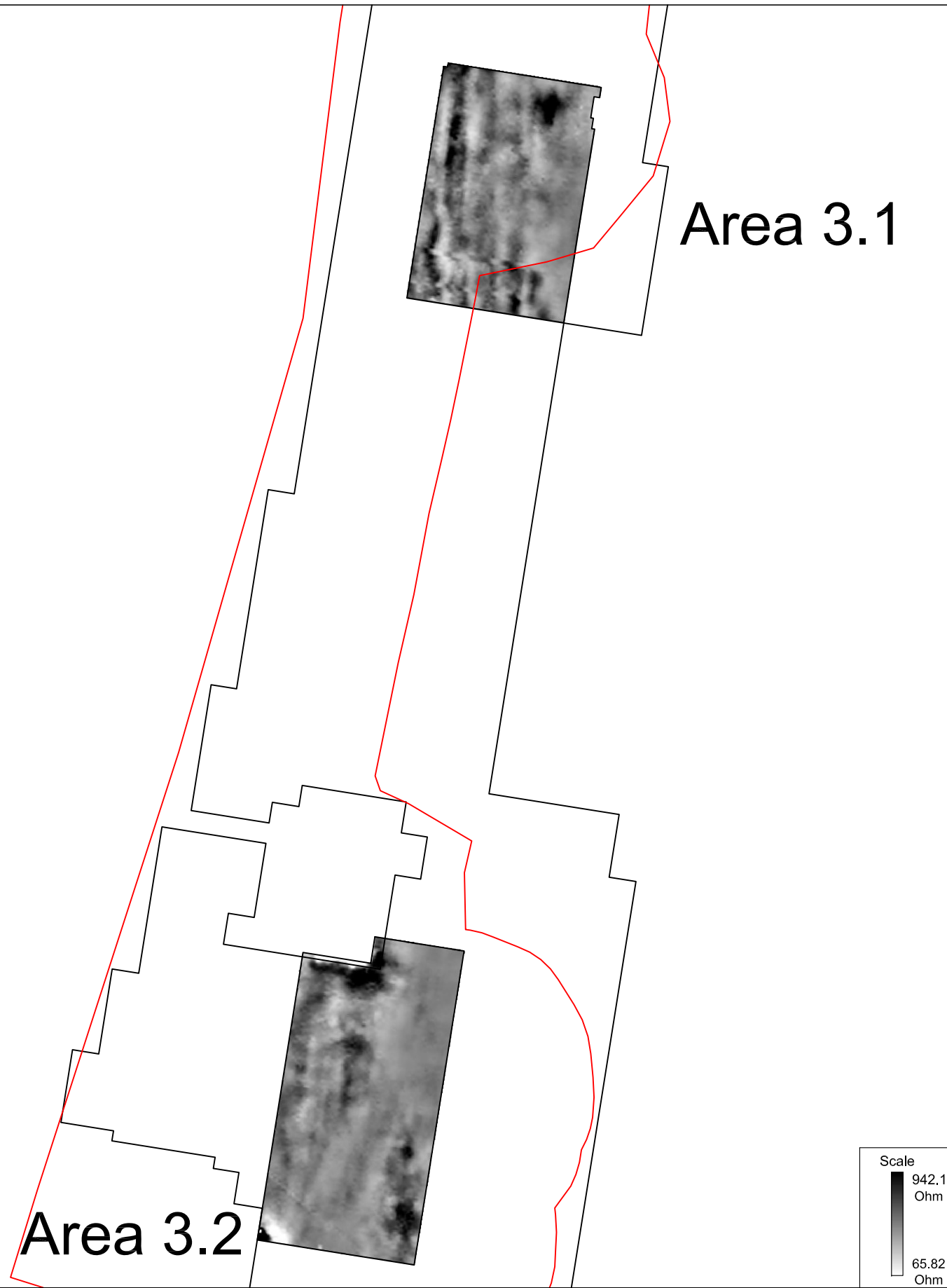
Processed Earth Resistance survey results - Area 3
