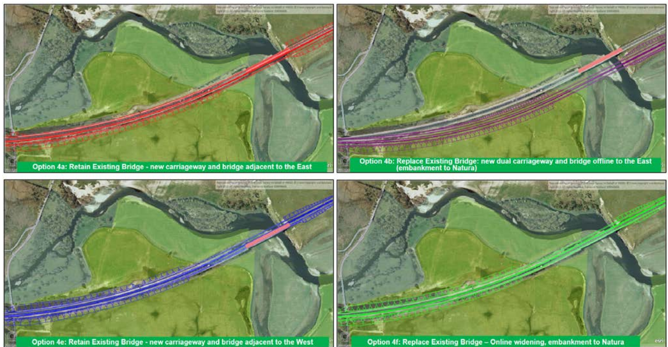
Figure 3-3: DMRB Stage 2 Options 4a, 4b, 4e, 4f at the River Spey Crossing
