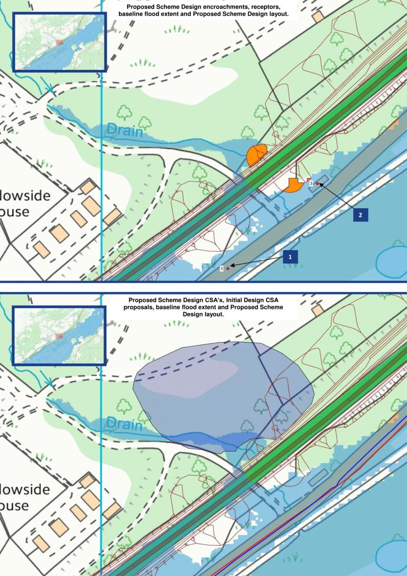
The introduction of a headwall around the Highland Wildlife Park access road crossing has reduced the encroachment on the upstream and downstream side.
