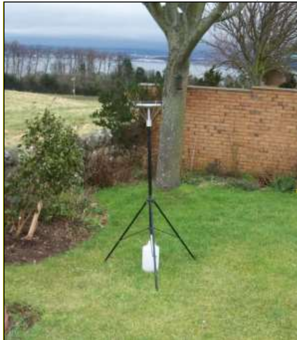
Figure 1: Example of an Installed Frisbee Gauge Meter
