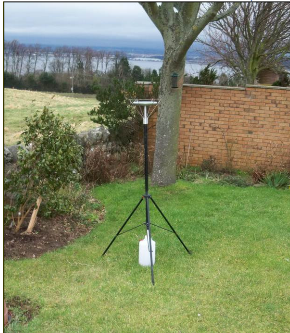
Figure 1: Example of an Installed Frisbee Gauge Meter
