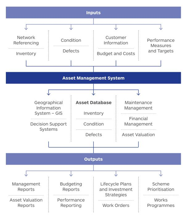
A key component of this is our Integrated Road Information System (IRIS), a Geographical Information System (GIS) map-based asset management system linking condition data with inventory, accidents, structures, drainage, construction, customer services, routine maintenance, works ordering/payment and street lighting. By managing our data more efficiently in this holistic way it enables improved investment decisions.
