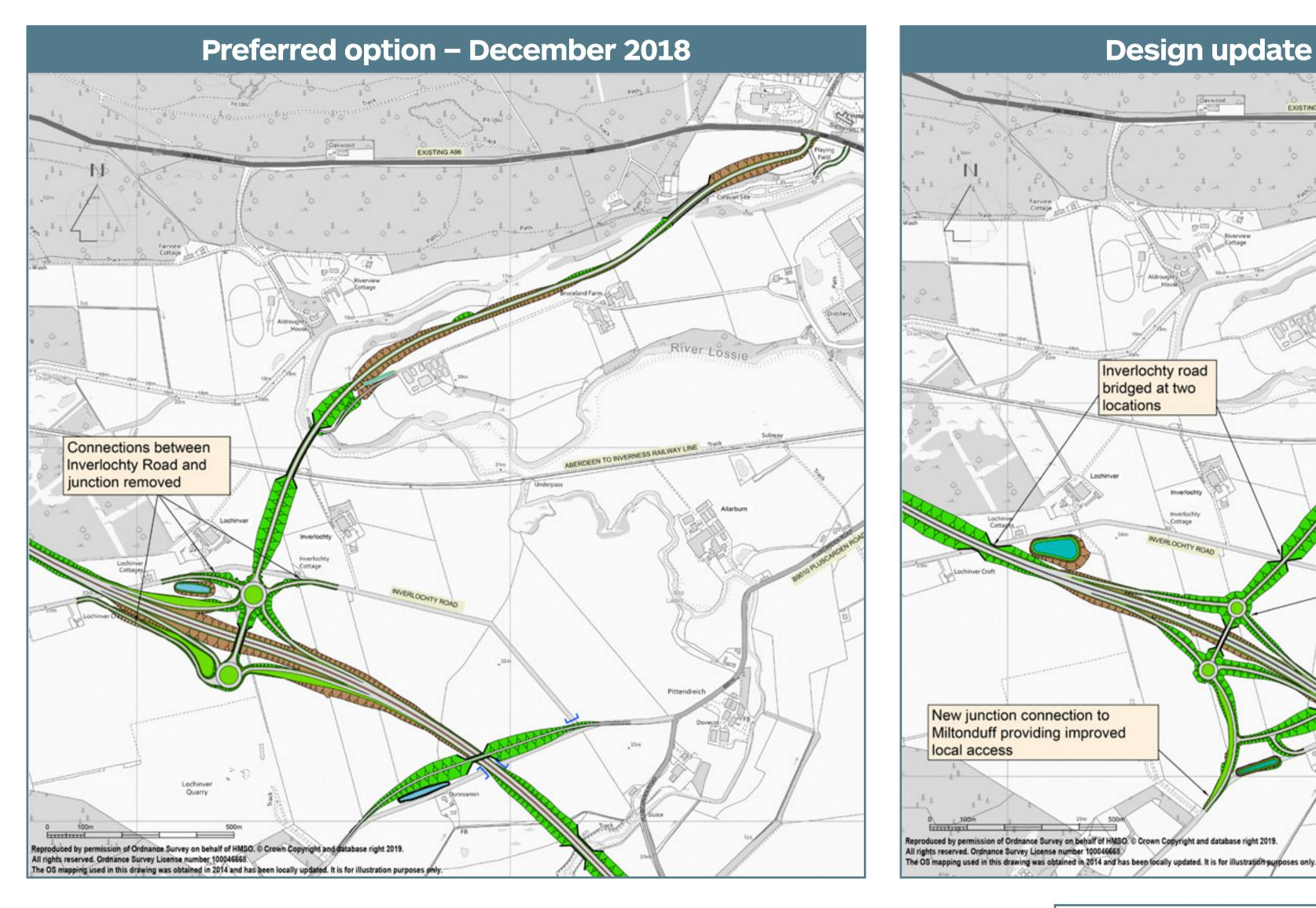
**OVERVIEW:** The updated design has improved local connections, reduced agricultural land loss, resulting in less farm fragmentation, significantly reduces effects on residential visual receptors, the grade-separated junction location fits better within the landform and provides greater value-for-money.
