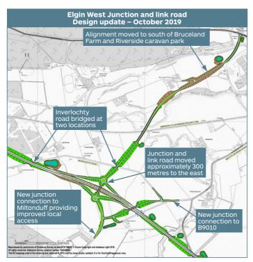
**OVERVIEW:** The updated design has improved local connections, reduced agricultural land loss, resulting in less farm fragmentation, significantly reduces effects on residential visual receptors, the grade-separated junction location fits better within the landform and provides greater value-for-money.
