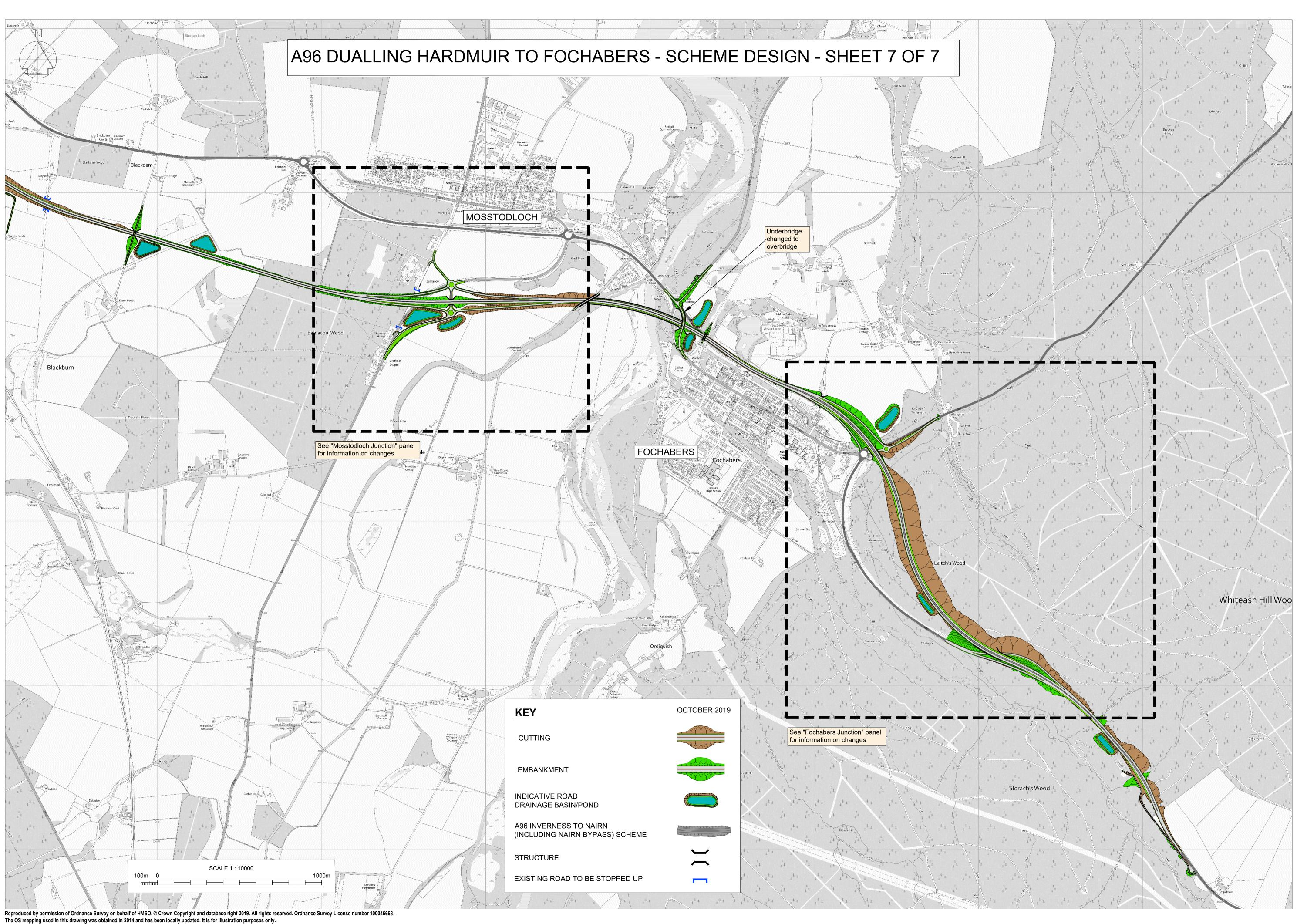
The scheme design and junctions shown have been designed using more recent survey information. The scheme design and junctions will be subject to further design and development as the scheme progresses.
